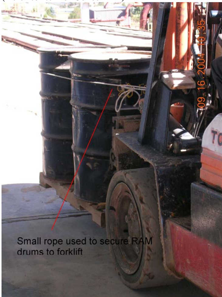
Image 5. Inadequate securing and movement of drums containing radioactive material. (Refer to Item of Concern #4)
