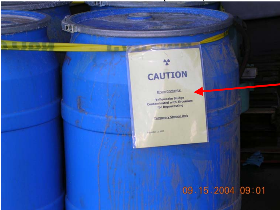
Image 1.2 Close-up photograph of drum containing radioactive material not posted in accordance with RH 4.30. (Refer to Item of Non-Compliance #1).
