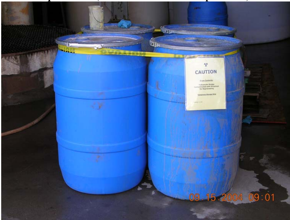
Image 1.1 Photograph of 4 drums containing radioactive material not posted in accordance with RH 4.30 requirements. (Refer to Item of Non-Compliance #1).
